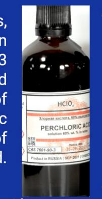
Brief description of the danger of perchloric acid: a strong oxidizer; may cause fire or explosion, may cause corrosion of metals, chemical burns if it gets on the skin.
